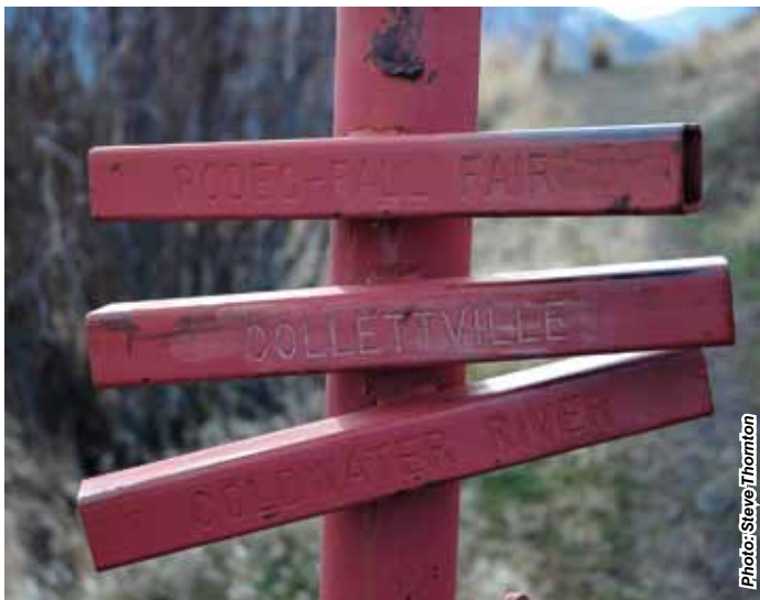
Sight tubes are labeled with the landmark visible by looking through the tube.
